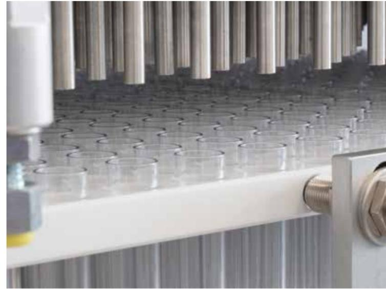
^ Drying additives in blood collection tubes. Based on the OPTIMA BCT-200, Optima Automation is able to implement a wide range of customer-specific requirements for both assembly and manufacturing processes.
