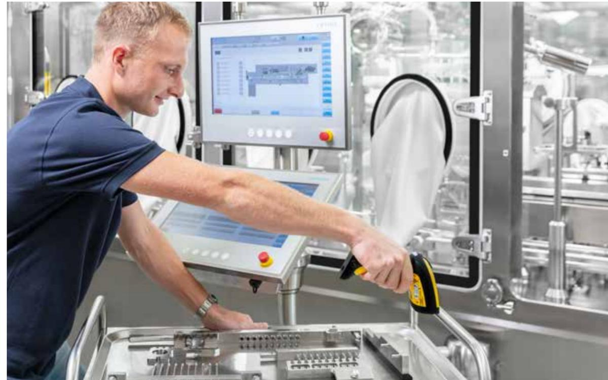
← Remote Support: Optima experts support operators via video and audio transmission for troubleshooting, format changes and maintenance work.
