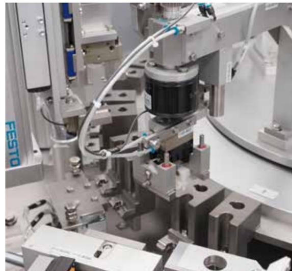
All processing stations are integrated on the rotary transfer machine. Here the knob of the dosing mechanism is turned back to the starting position.
