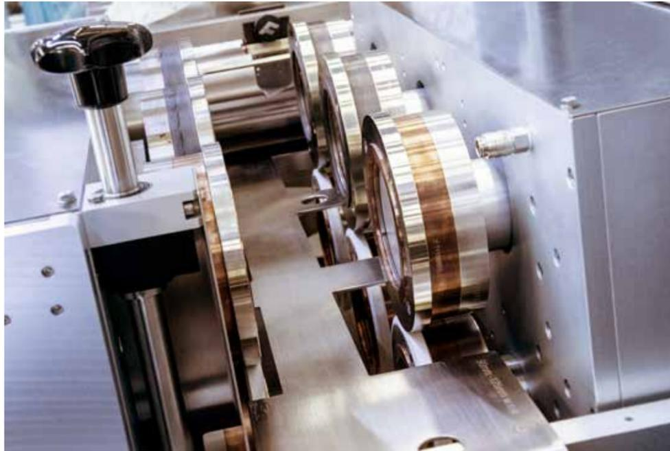
Sealing station: The four-sided sealed pouches are sealed in a continuous process.
