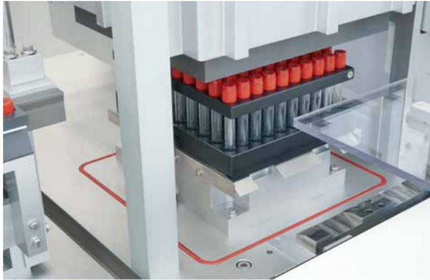
^ The OPTIMA BCT-200 assembly line manufactures and packages blood collection tubes. Additives are dispensed into the tubes, which are then vacuum sealed.
