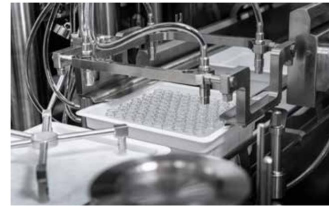
After removing the Tyvek foil and the cover, the syringes are brought into the processing position.
