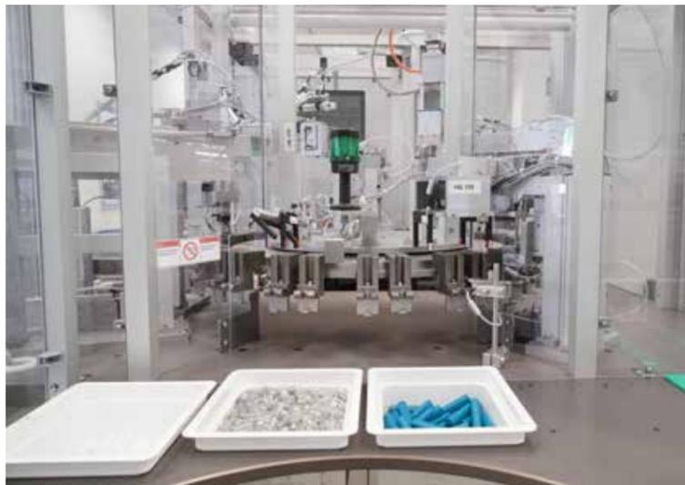
After the components have been manually inserted, the automated assembly process starts. The machine design can subsequently be adapted to be fully automated.
