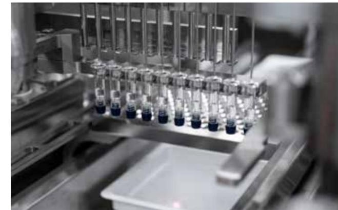
High output of up to 36,000 pre-filled syringes per hour: Rotary piston pumps ensure dispensing with a ten-head concept. Additionally, Adimmune can put a peristaltic pump system into operation.
