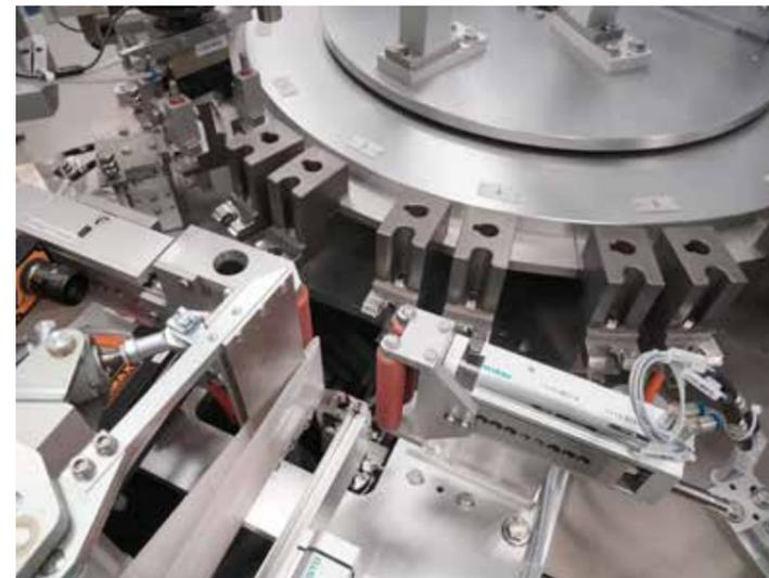
The dosing mechanism of the pen is pressed in at this station.
